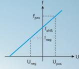
The frequency shift produced by the Bragg cell makes the fringe pattern move at a constant velocity. Particles which are not moving will generate a signal of the shift frequency  $f_{\text{shift}}$ . The velocities  $U_{\text{pos}}$  and  $U_{\text{neg}}$  will generate
